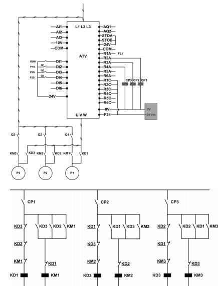
Each pump is controlled by a relay output:
