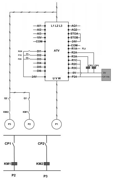
Pump 2 and pump 3 are controlled by relay outputs R2 and R3.
