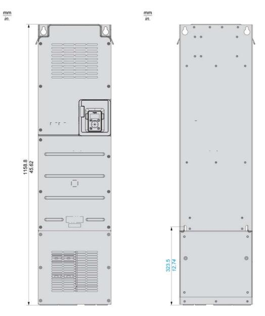
IP20 Drives - Rear, Front and Side View With Top Cover and Conduit Box
