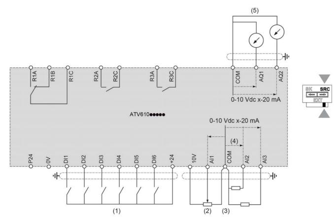
(1) Digital Inputs - Shielding instructions are given in the Electromagnetic Compatibility section *(see page 71).*
